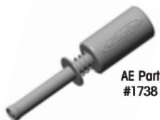
**Glow Plug Starter** The glow plug starter is a battery powered device used to heat up the glow plug so the motor will start up. Once the motor starts, the glow plug starter will be removed.
